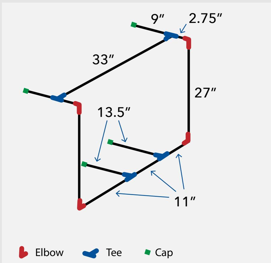
3. Use the PVC cement to secure the PVC sections into the connectors (elbows, tees, and caps). Follow instructions on the PVC cement packaging for proper use.
