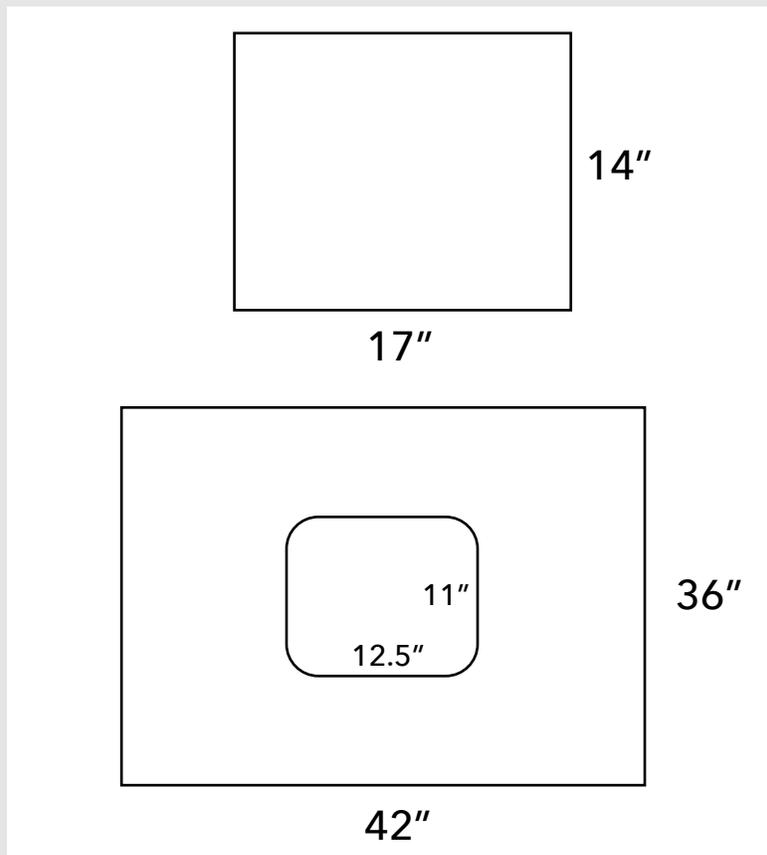
5. Attach the 42" x 36" vinyl piece to the PVC by sealing it around the vertical 27" sections. Lay the vertical PVC section on top of the vinyl and fold ~2-3" of the vinyl over the PVC, creating a pocket for the PVC to sit in. Use an impulse sealer (or another heat source like an iron) to seal the vinyl around the PVC.
