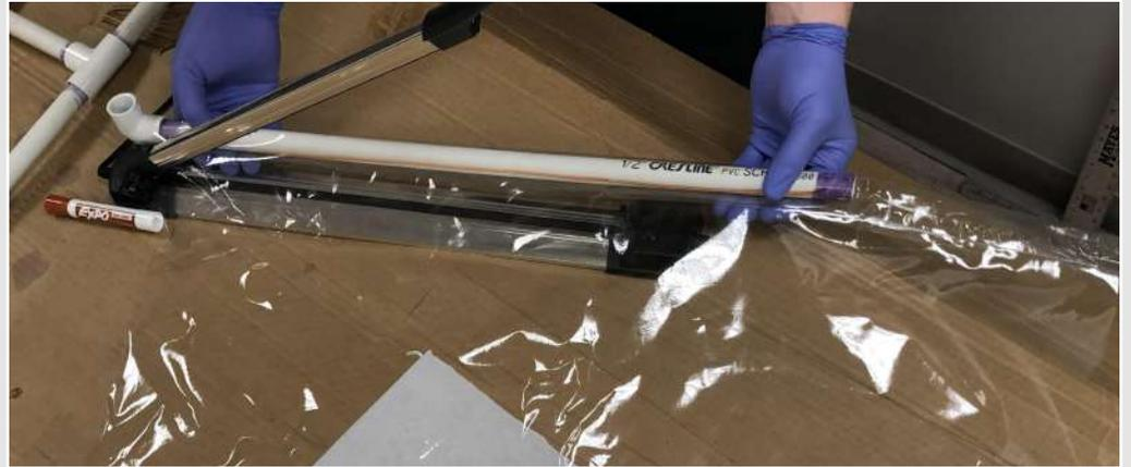
6. Pull away the plastic so that you can place a piece of 2" wide double-sided tape in the locations shown in the drawing below (denoted by a T).
