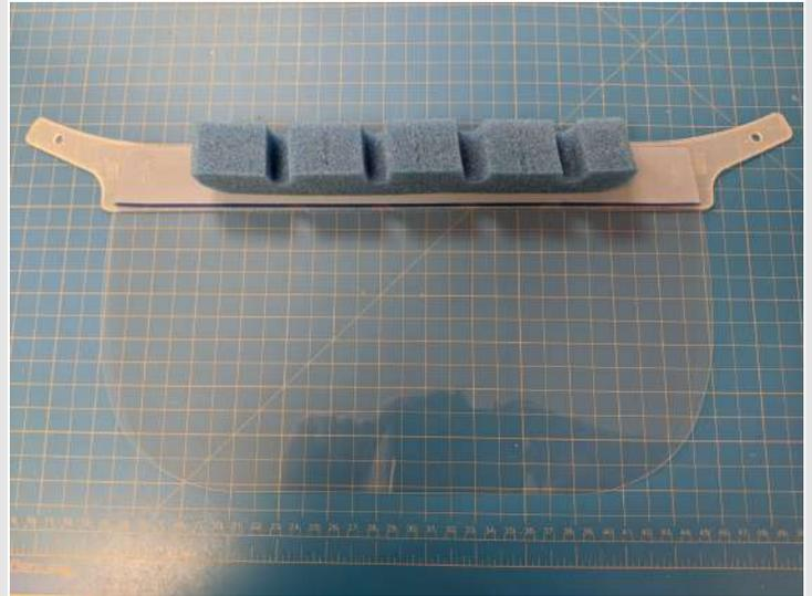
5. Disassemble the screw assembly on either end of the welding headgear. Attach the headband-faceshield assembly from Step 4 onto the screw on either end of the welding headgear. Make sure the foam piece on the headband is facing inside.
