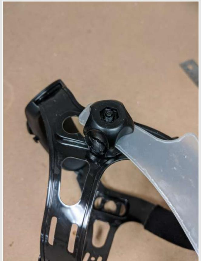
6. If you ever need to replace the faceshield, you can detach from the support band and replace with a new one by following Step 4.
